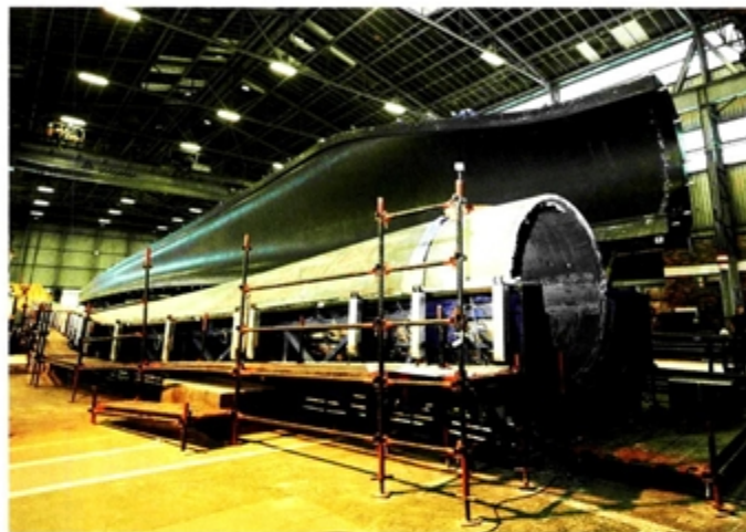
I-WEC's 50 metre long wind turbine rotor blade is exposed as the mould it was made in is opened and it is lifted out for the first time
